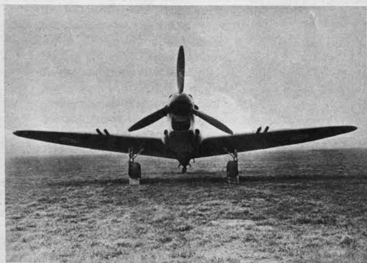
FIREFLY Replacement for the Fulmar, the Firefly is a long-range fighter, reconnaissance plane and nightfighter. Head-on view shows one big and four small air intakes under the Rolls-Royce
